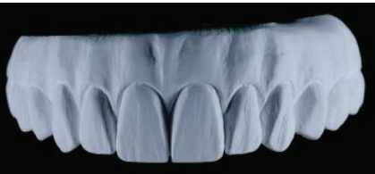
Above: First stage of green state – Initial refining of milled green state zirconia. Photo and case by Vadim Vainer, Shiksha Dental Laboratory.
